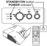
However, to maintain better picture quality, the lens door will close after the lamp has been cooled down when the projector is installed upside down such as in ceiling mount installation. Then the **POWER** indicator will stop blinking and light in steady orange when the lamp cooling is complete.
